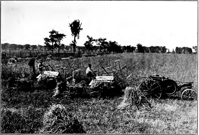
HARVESTING TO-DAY. A Mogul Kerosene Tractor pulling two McCormick reapers and binders with mechanical shockers. The tractor is managed by the man on the front reaper. Two men take the place of six human beings in the previous cut and do many times as much work, in much greater comfort. This, of course, is a development much later than the Civil War.
